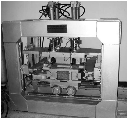
Fig. 4. A large-scale test device of the interface, CSASSI [22].
